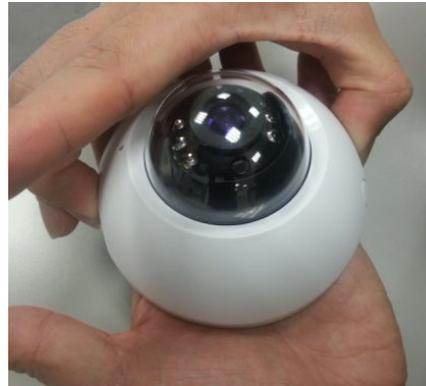
c. Unscrew the lens for adjust the angle.
