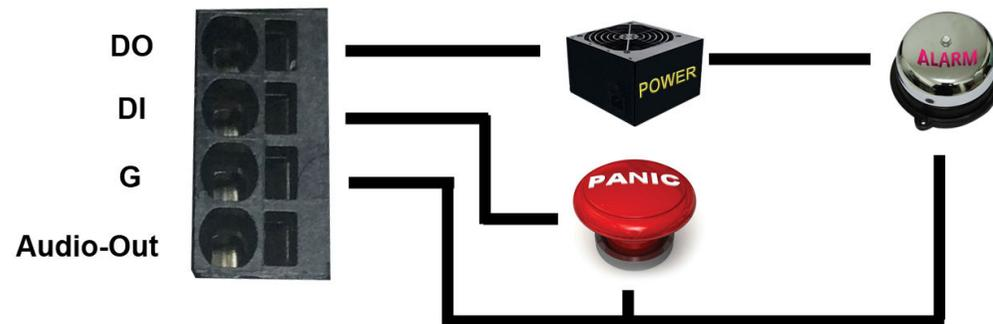
When no event occurs, the DO output is 5V (DO and GND are disconnected). When the camera detects events it will trigger and external alarm, DO output is 0V (DO and GND are connected).
