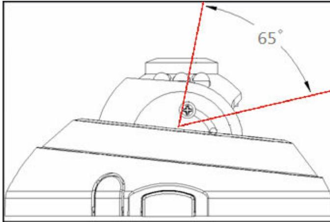
d. After adjusting the lens tight the screw. Repeat steps b & C as many times you need during the whole process.
