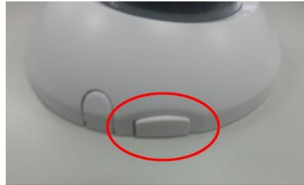
b. Use screws to place the bottom of camera to the ceiling or the wall. **Do not lock it completely because you might need to adjust the lens angle later.**
