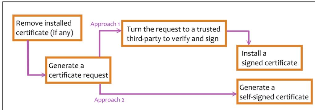
Remove the existing certificate: Before you generate a new certificate, please remove the installed one. Select the **Http** connection type and click **Remove**. If a dialog box pops up to ask you to confirm, click **Yes**.
