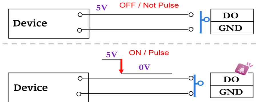
If you select **N.O** on **Input sensor setting**, when the switch contacts are opened, the camera input alarm will be triggered and will execute the action user has set, for example, send a snapshot to E-mail address.
